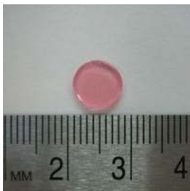
Figure 8. 2% agarose disc (8 mm in diameter and 2mm in thickness)
